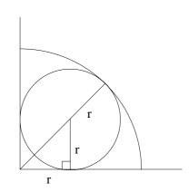
From the diagram, if r is the radius of the circle then the radius of the quadrant is r  $(1 + \sqrt{2})$ .
